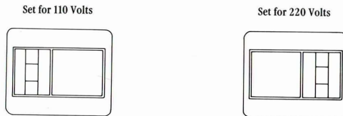
Figure 1-4. Computer Line Voltage Settings
